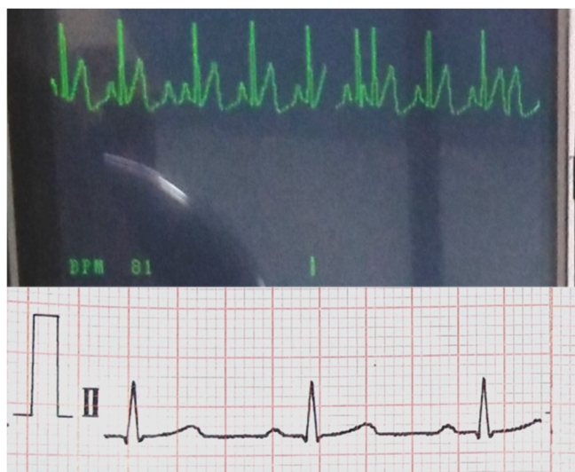
FIGURE 11. ECG graph on the TFT Module and on the Comparison ECG with phantom leads with a setting of 80 BPM
