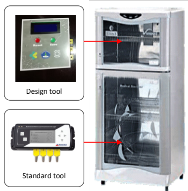
FIGURE 3. In order to test the research module, a comparison test was carried out using a comparison tool. As many as 9 Sensors from the research module and the comparison module were placed close to each other in the sterilizer
