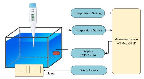
FIGURE 1 The block diagram of Digital Wet Media thermometer calibrator, input temperature sensors, is processed by a ATMega328P minimum system. Result of the temperature reading will be displayed on the 2x16 LCD to display. Heating was carried out in an ideal room and is controlled using PID control.
