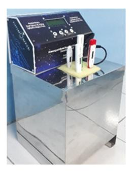
Figure 3. Research results module. The module was designed to make it easier to place the thermometer to be tested. The display of the measurement results can be seen on the LCD
