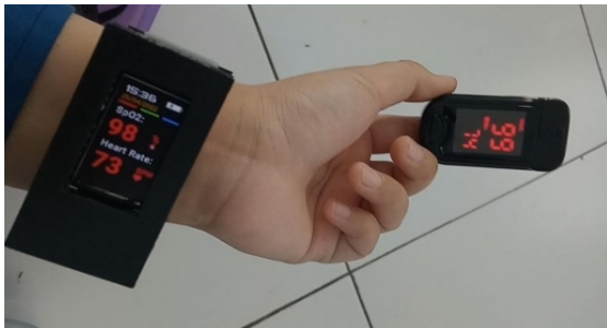
FIGURE 2. The process of measuring BPM and SpO2 parameters using Smartband module design and pulse oximetry (Finger Pulse Oximeter General Care Model F02T)
