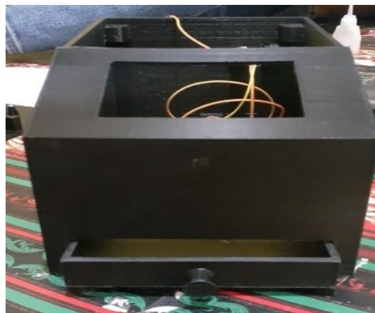
FIGURE 6. The proposed design Safety Device Ultra Violet Light for Mercury Identification in whitening cream with thin layer chromatography method using camera OV7670 based on Arduino Uno
