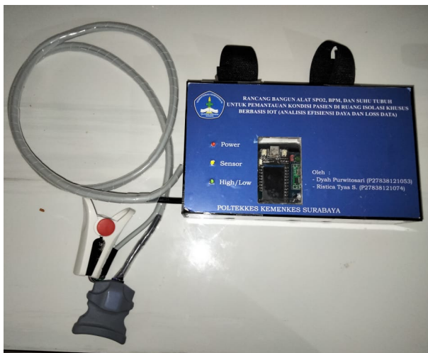
FIGURE 3. Design and build a patient condition monitoring tool in a portable form. Consists of 3 parts, namely the MAX30102 and MCP9808 sensors, cables, and the main part (ESP32 TTGO, indicator LED, and battery).
