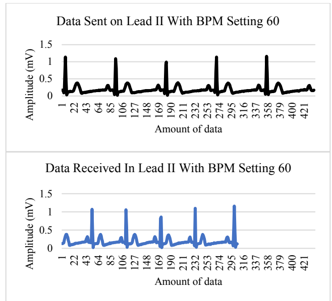
FIGURE 4. Data Comparison of Sent and Received ECG Lead II Signals At 60 BPM
