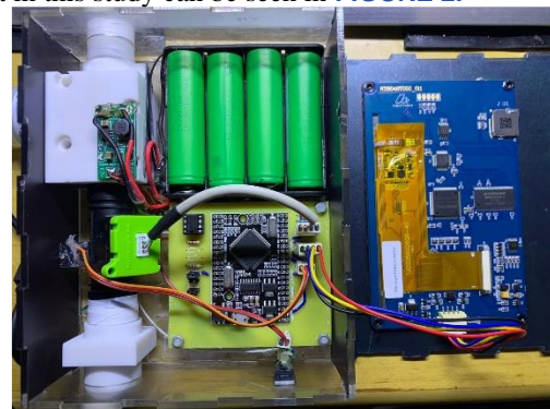
FIGURE 2 . Overall circuit design in research on high flow oxygen analyzer
