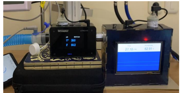
FIGURE 1 . Gas Flow analyzer Citrex H3 When Measuring the High Flow Oxygen Analyzer on the oxygen concentration setting
