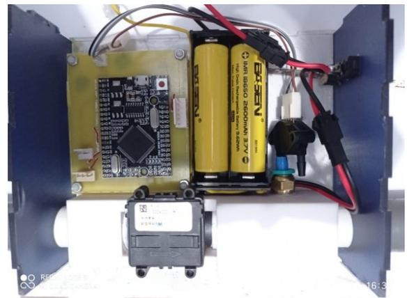
FIGURE 3. overall circuit ventilator tester using sensor F1031V
