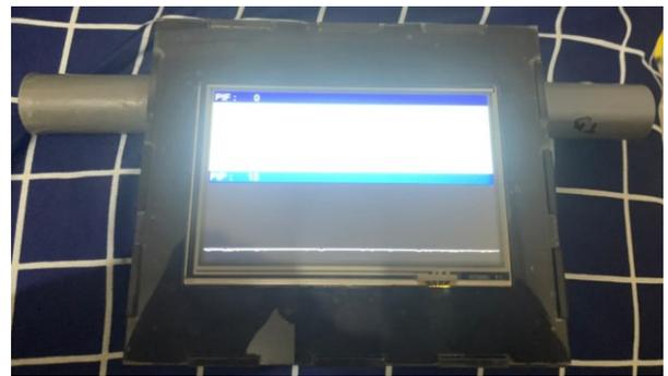
FIGURE 2. Ventilator Tester Display Ventilation Tester display with two PIP and PIF waveforms for validation
