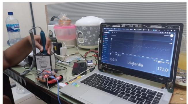
FIGURE 1 . Front View Module with experiments on a fetal heart rate simulator
