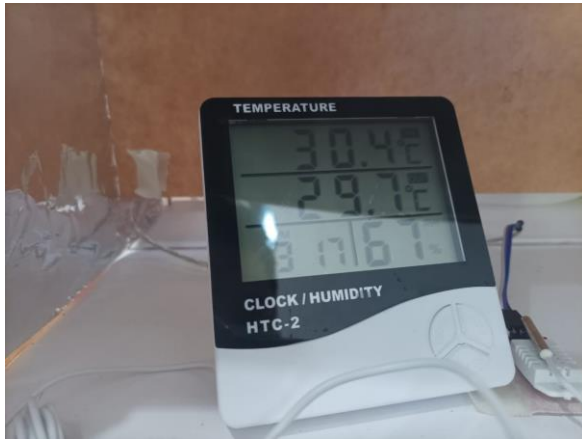
FIGURE 7. Testing the DHT22 temperature sensor using the HTC-2
