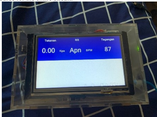
FIGURE 3 . Module view with pressure, RR, and Voltage display on TFT LCD
