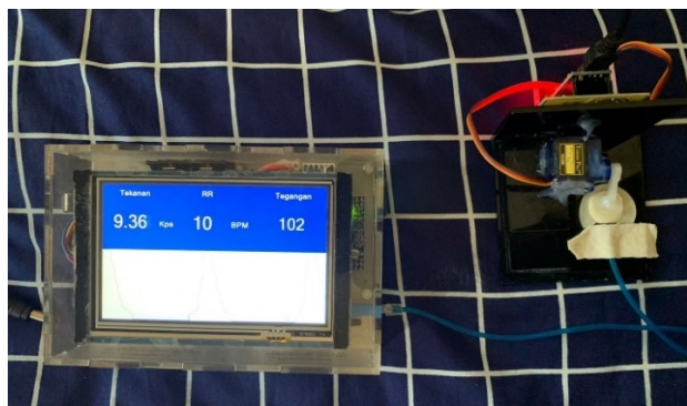
FIGURE 4 . Appearance of the module at the time of data collection using a servo motor simulator and abdominal respiratory sensor
