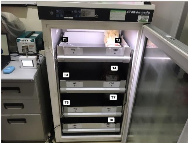
**FIGURE 3.** Location of measurement points T1, T2, T3, T4, T5, T6 dan T7 using the Blood bank.
