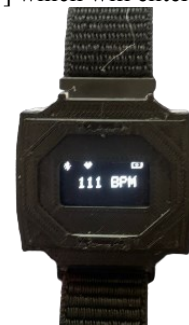
FIGURE 3 . Smartband module display with heart rate, body temperature and battery capacity display
