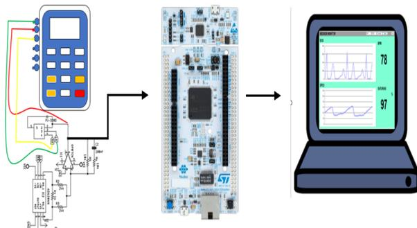
FIGURE 3. BPM testing diagram on a phantom
