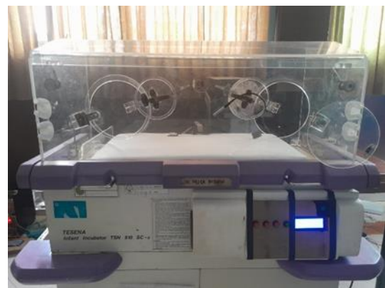
FIGURE 3. Modified module from the TESENA brand which is equipped with monitoring of temperature, humidity, and noise parameters through an IoT-based WiFi network.
