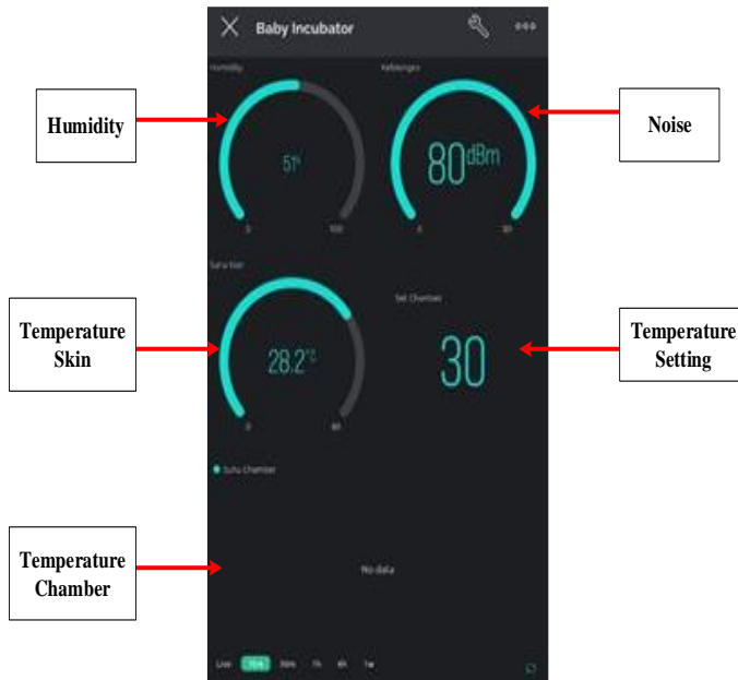
FIGURE 4. Results Display of temperature, humidity and noise parameters on android with blynk platform.
