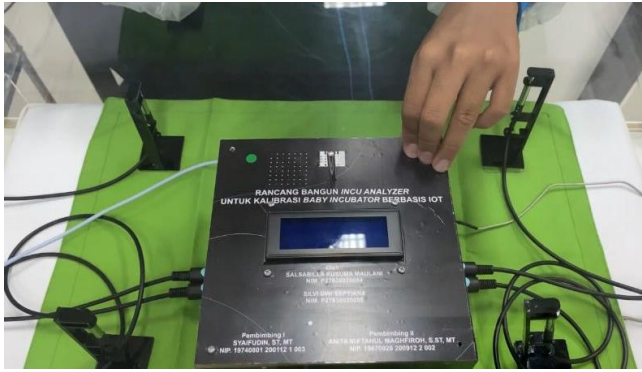
FIGURE 3. The Incu Analyzer module measures the chamber temperature of the baby incubator.
