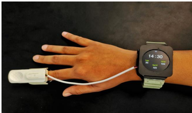
FIGURE 4 Smartband module display with heart rate, SpO2, and body temperature.
