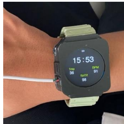
FIGURE 4. Smart band Module Design with MAX30100 Sensor and MLX90614 Sensor and using LCD TFT 1.28inch GC9A01A
