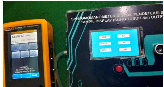
FIGURE 3 Calibration Using a Fluke brand DPM with measurements five times per setting
