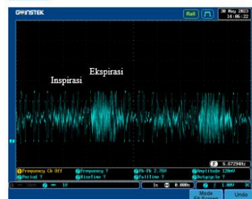
FIGURE 4 Pulmonary sound signal output after passing non inverting.
