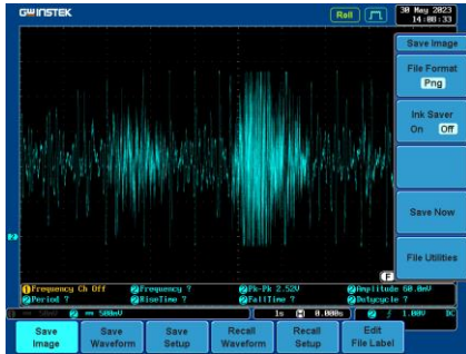
FIGURE 5 Lung sound signal output after passing non-inverting 2
