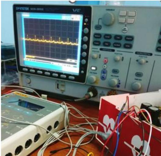
FIGURE 5. The results of the ECG signal display on the oscilloscope
