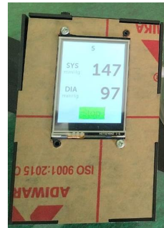
FIGURE 4. IoT Based Ambulatory Blood Pressure Monitoring Design. The results of the systole and diastole values are displayed on the display module.
